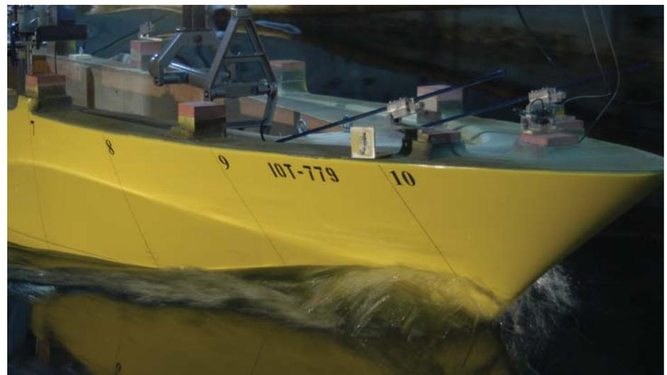
*Model during calm water resistance test.*
