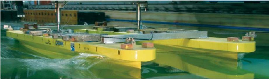
*Vancouver SeaBus in the 90-meter Towing Tank.*
