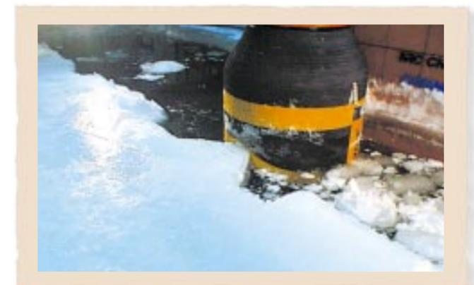
▲ Test of Ice Abrasion on Marine Hose
