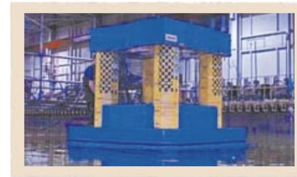
▲ GBS Model Ready for Testing in IMD Offshore Engineering Basin
