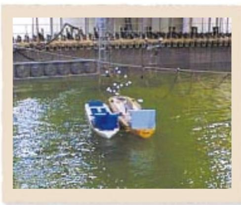
▲ Model Test of Side-by-side Configuration
